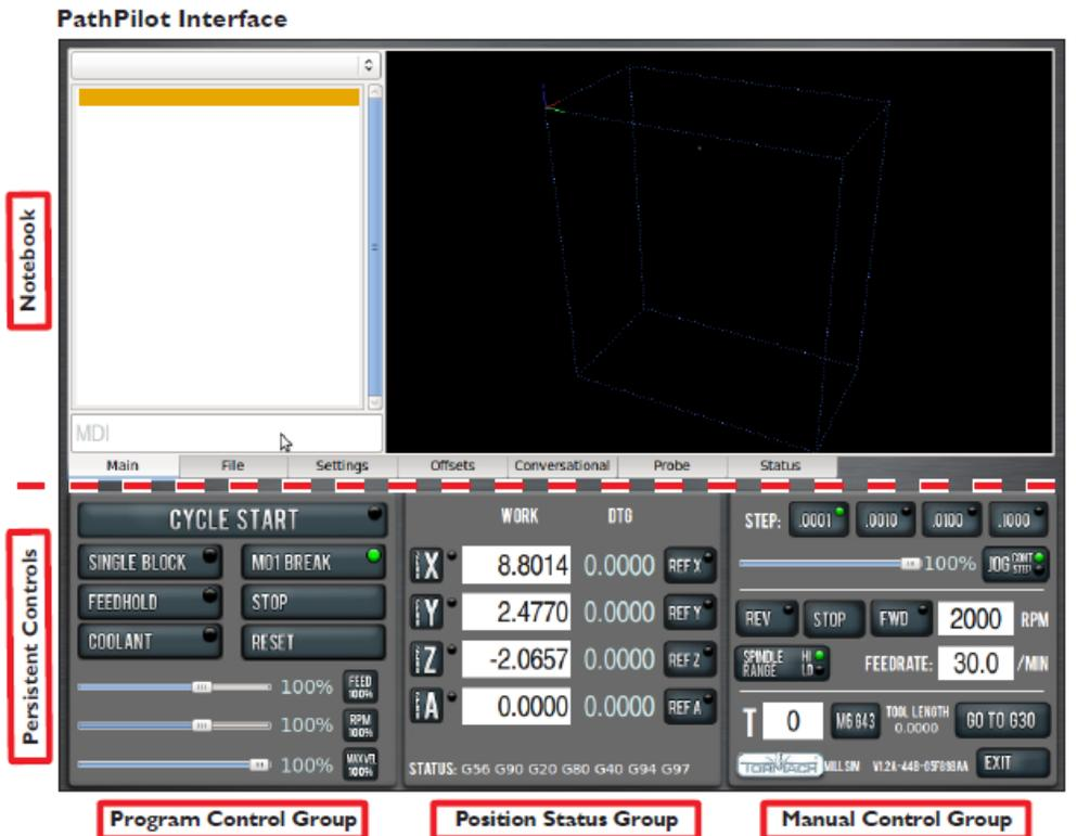
The PathPilot interface runs on the computer monitor located on the right side of the milling machine. Power to the computer must be turned on using the Controller switch on the Control Panel. In addition, the main power switch must be in the on position. You may also have to turn the computer's power switch on. Once the computer is booted, make sure PathPilot is running.
