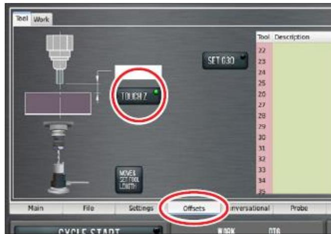
Verify the tool length in the tool description table and enter the tool diameter.
